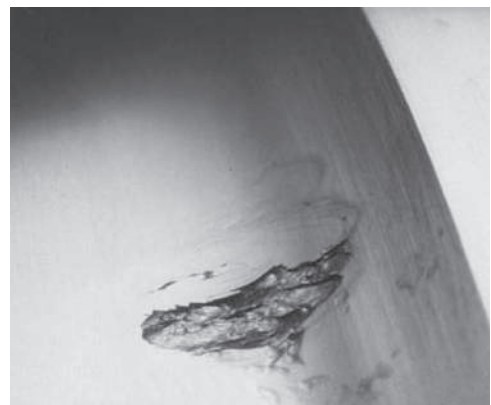
Fig. 5.2 Photo-illustration of fatigue damage on the raceway
